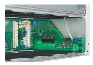
The BCC is a system supervisory module that provides basic control and monitoring functions for the Intergy Series Mini Power Systems. It is the ideal solution for systems where only minimum control and alarm features are required.
